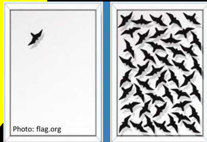
Ineffective versus Effective Window Decal Application
